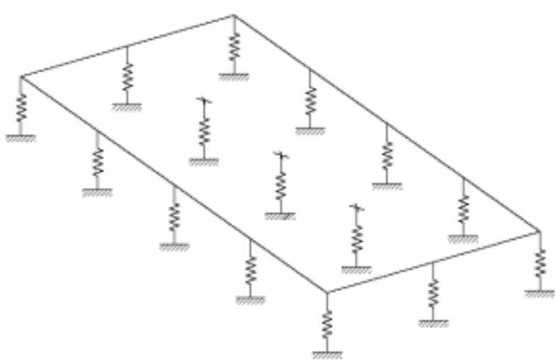
Figure 10.6 The coefficient of subgrade reaction forms the basis for a "bed of springs" analogy to model the soil-structure interaction in mat foundations.
